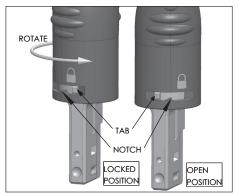
Figure 2: Removing the Magazine Cover
